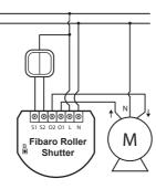
Fig. 1 Roller Shutter wiring diagram
