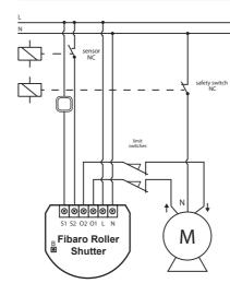
Fig. 2 Connecting Roller Shutter to GATE motor
